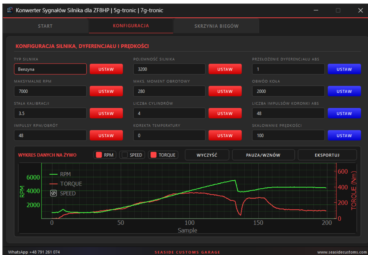
Engine, differential and speed parameters plus the live data chart
